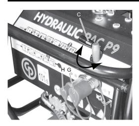
The by-pass valve (C) must be in the OFF position when starting and in the ON position when using the machine.
