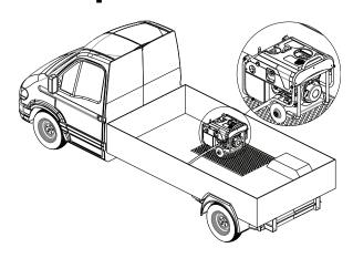
During transport make sure the power pack is secured. Ensure that the power pack is upright during transportation and lifted with approved lifting equipment.
