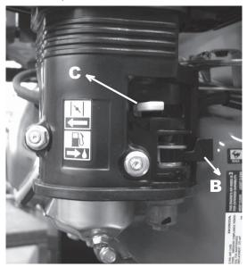
3. Move the choke control (C) to the CLOSE position. If the engine is warm, or the air temperature is high, move the choke control to the OPEN position.
